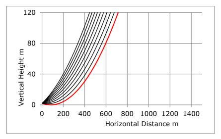
8.3 In the second case the noise source is at 80m and the turbine can be heard upwind up to about 500m. Note that in the space to the left of the red line and the Y-axis the listener will receive the direct sound down form the noise source.
