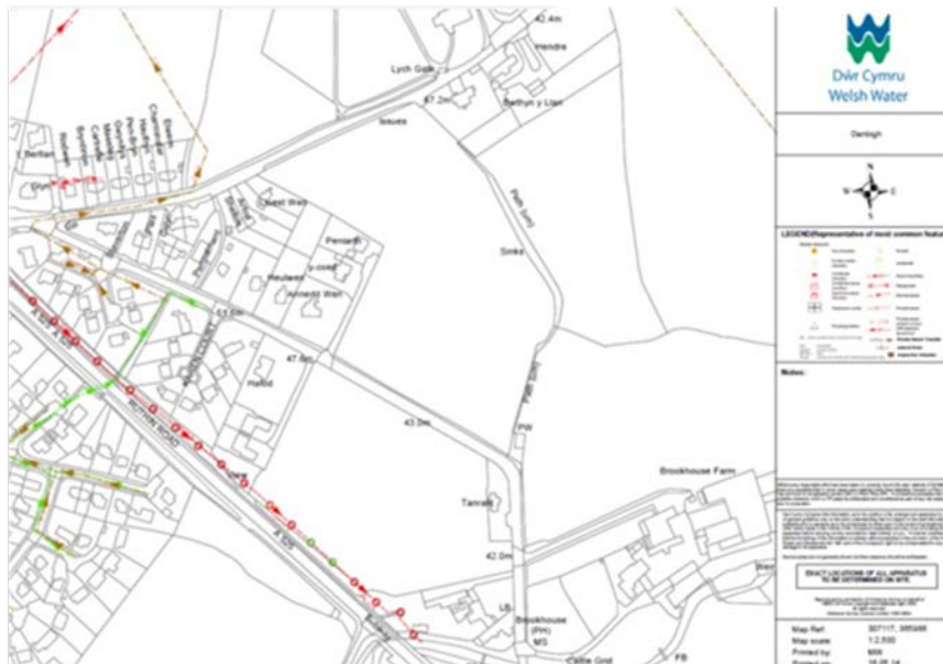
Figure 10: Local water and sewerage network
