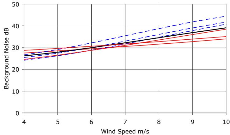
2.7 Particularly around 6m/s – which is the wind speed at which turbine noise usually exceeds background noise by the largest margin, the noise levels are very close. Furthermore the average line is similar to the average of a large number of measurements I have seen that have been taken in rural areas.
